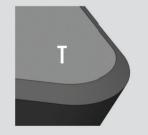
CHAMFER / T-LAND: The larger the T-land width and angle, the higher the forces
